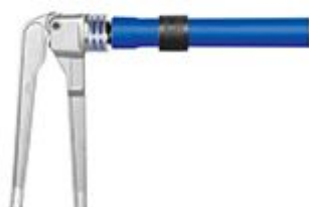
2. Expand the pipe twice (offset by 30°)
