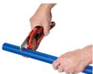
1. Cut pipe at right angles
